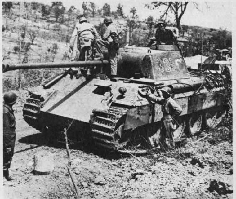
Star performer in Normandy, the Panther mounts an 18-ft. high-velocity 75-mm. gun. Broad track is supported by overlapping wheels.
